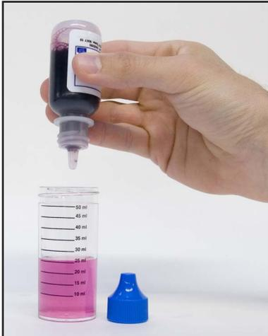
**4** Add Hardness Titrant drop-wise, while swirling, until the sample color changes from red to blue. Record the number of drops.
